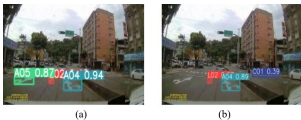
Fig. 6. YOLOv8 missed to segment the class A05. (a) YOLOv5. (b) YOLOv8.
